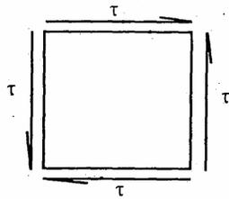
The above figure shows the stress condition of an element. The principal stresses are
