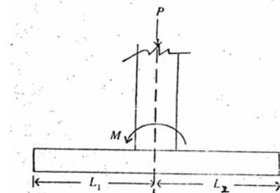
A rectangular reinforced concrete footing is to be designed to support a column which transfers axial load and uniaxial moment to the footing as shown in the above figure. The footing is to be designed to have uniform upward soil pressure. The dimensions  $L_1$  and  $L_2$  ( $L = L_1 + L_2$ ) of the footing would be
