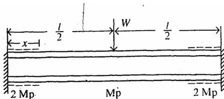
For a fixed beam shown above, it has been decided to weld coverplates at ends so that moment capacity doubles at the ends. If maximum advantage has to be derived, the length  $x$  of the plate should be
